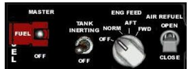
Next to it is the **fuel pumps control switch**. This has 4 positions:
