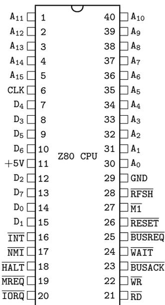
**A<sub>15</sub> – A<sub>0</sub>** *Address bus* (output, active high, 3-state). This bus is used for accessing the memory and for I/O ports. During the refresh cycle the IR register is put on this bus.
